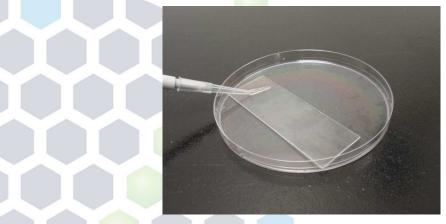
Carriers were inoculated with 0.020 ml and the test inoculum was spread to cover a surface area of approximately 15 cm<sup>2</sup> (and to within  $\sim$  3 mm distance from the carrier perimeter).
